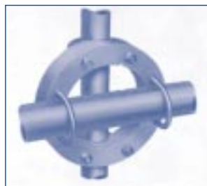
Pt. No. 9637875 Heavy Duty Cross-over Clamp for connecting booms of 29-51mm at right angles to 29-51 O.D. tubular masts. For connecting up to 76mm O.D. tubular masts specify Pt. No. 9638068
