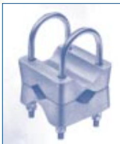
Pt. No. 9637423 Cross-over/Parallel Clamp for connecting booms of 29-51mm diameter to 29-51 O.D. tubular masts
